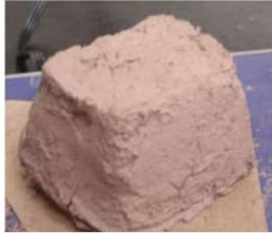
▲ Muestra seca, 318,5 cm<sup>3</sup>
